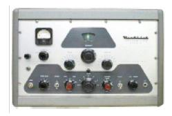
Kit builders in the 1960s often built entire ham stations from the Heathkit line. Phone ops often chose the DX-100 transmitter. It was truly a "big bertha," weighing 100 pounds, and delivering 125 watts of AM and 140 watts on CW. It covered 160 to 10 meters with VFO or crystal control.
