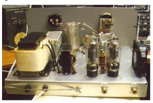
**Firing it up:** Joe's amplifier passed the "smoke test" handily. "I checked it out on a dummy load with an oscilloscope and verified that it was linear and had no flat topping." His first QSO was on the 75-meter 'Boat Anchor' net.
